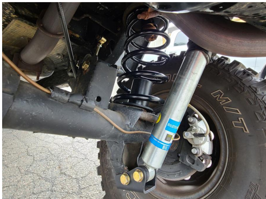
Figure 3: Spring reinstalled in spring perch
