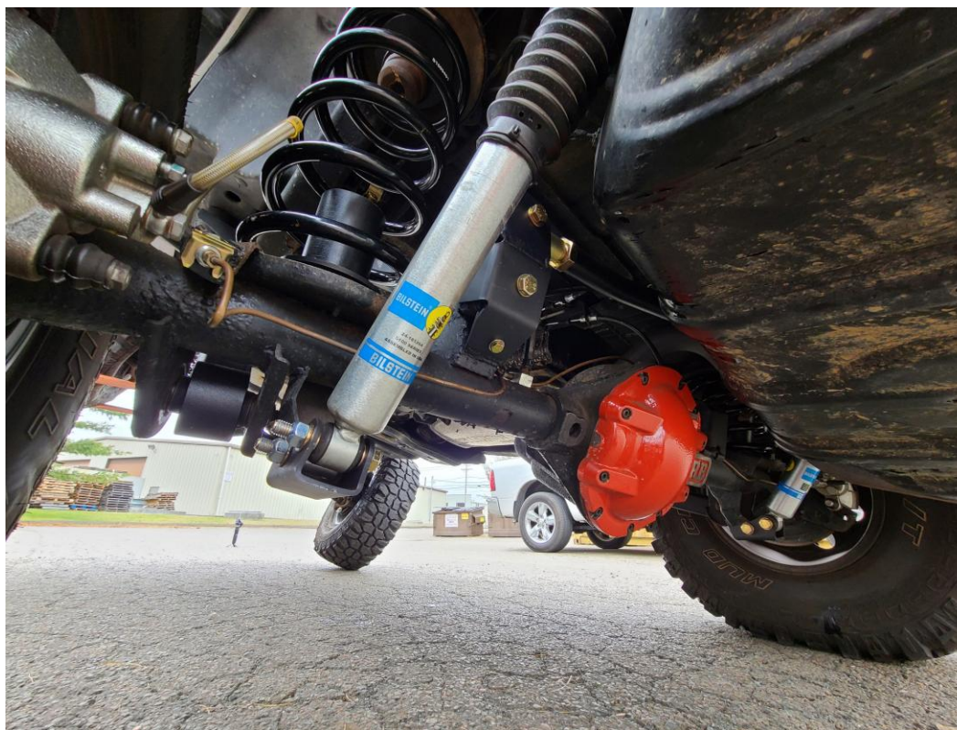
Figure 4: Rear track bar reinstalled at the axle mount
