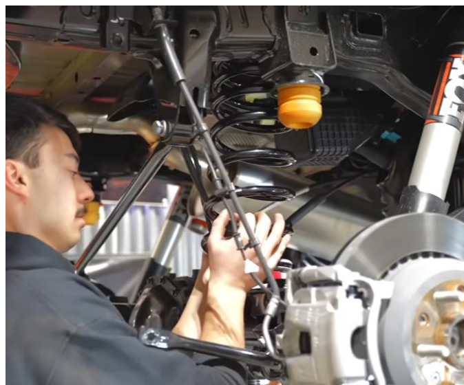
Figure 25: New, side-specific springs replaced
