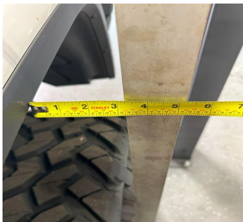
Axle track (rear driver side)
