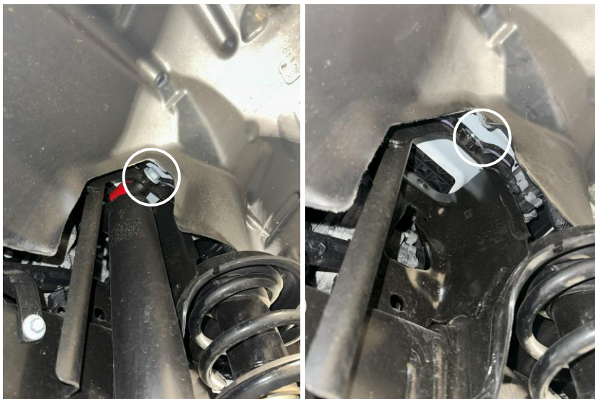
Figure 5: Front upper passenger shock bolt removed
